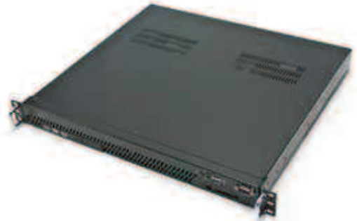
Intel Core2 Duo 3.0GHz, 2Gb RAM, 60 Gb solid-state hard drive. Certified to IEC60945. One Unit high (1.75") 19" rack-mount case with brackets. Measures 433 x 390 x 45mm excluding brackets. Weight 6.8 Kg.
